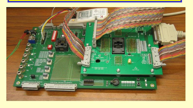
Digital logic under development on FPGA (Wang, Kroseberg), will be included on front-end ASIC after performance verified on test bench and in test beam.
