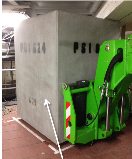
Concrete container from PSI to permanently house the spent target
