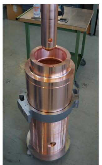
Two series cavities (QP2 and QP3) produced at CERN have been coated
