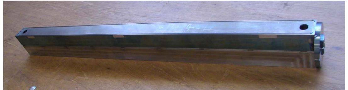
Dry (stainless steel) RF load
