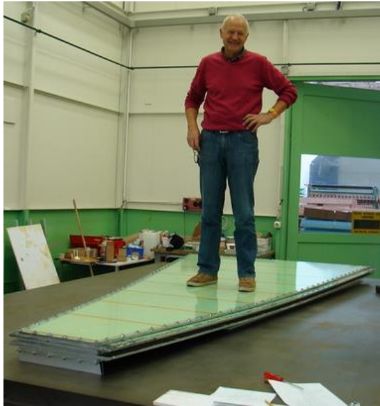
nSW Micromegas sector-sized prototype fully assembled. Study panel deformation and sag, measure elastic & mechanical properties.
