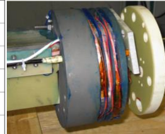
Cable channel filled with Stycast underneath conductor
