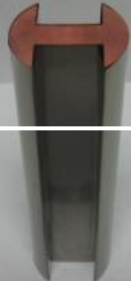
EDM Channel with Ti Etching Barrier in Billet Assembly
