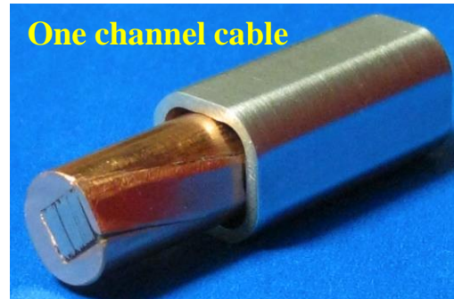
Cross-section and a twisted stacked-tape conductor
