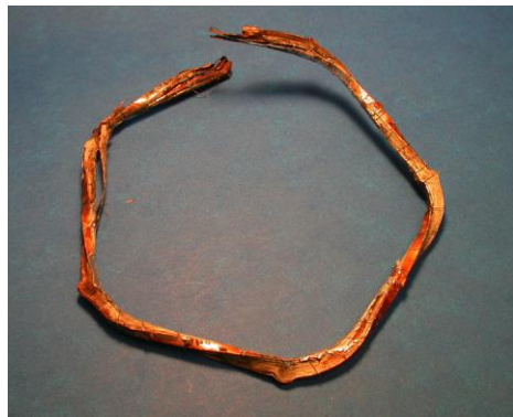
Damaged by Lorentz load.
