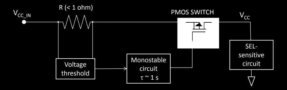
When a SEL-sensitive circuit develop a SEL, it draws more current. An external circuit can detected this situation and cycle the power.
