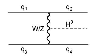
$$\begin{split} &\sigma(fa\to f'X)\approx \int dx dp_T^2 P_{V/f}(x,p_T^2)\sigma(Va\to X) \\ &P_{V/f}^T(x,p_T^2) \; = \; \frac{g_V^2+g_V^2}{8\pi^2} \frac{1+(1-x)^2}{x} \frac{p_T^2}{\left(p_T^2+(1-x)M_V^2\right)^2} \\ &P_{V/f}^L(x,p_T^2) \; = \; \frac{g_V^2+g_V^2}{4\pi^2} \frac{1-x}{x} \frac{\left(1-x\right)M_V^2}{\left(p_T^2+(1-x)M_V^2\right)^2}. \end{split}$$
