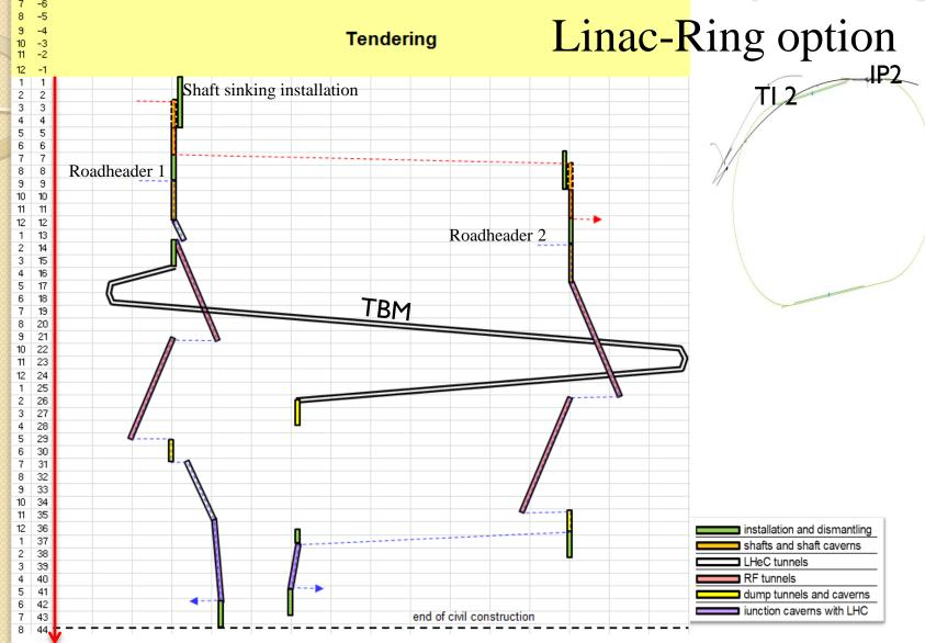
3.5 years for underground works using 2 roadheaders and I TBM
