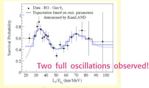
oscillations driven by  $\delta m^2 \sim 7.6 \times 10^{-5} \text{ eV}^2$
