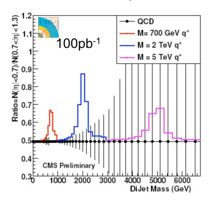
Small systematic due to use of ratio: Di-jet Ratio =  $N(|\eta|<0.7) / N(0.7<|\eta|<1.3)$
