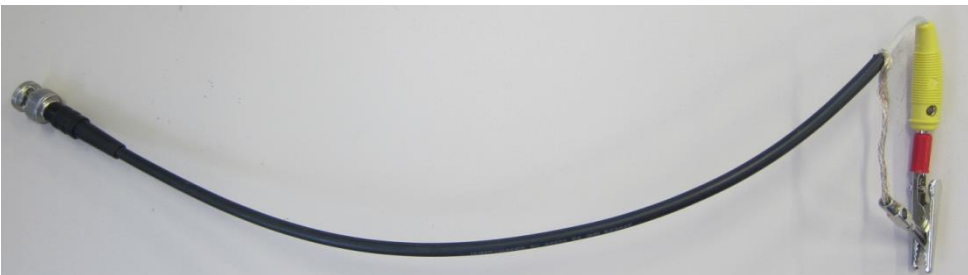
The makeshift loop antenna for system-external measurements
