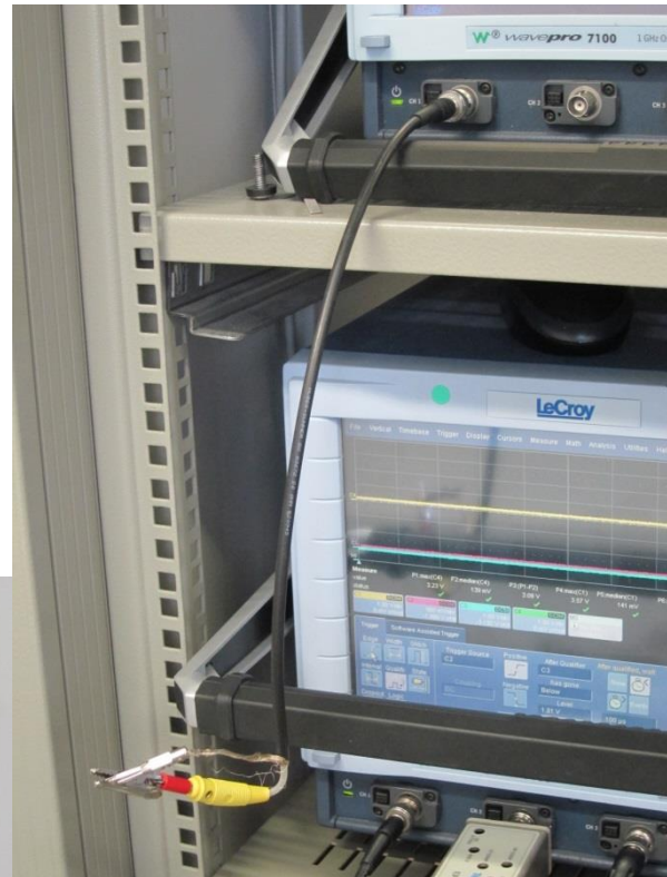
The makeshift loop antenna for system-external measurements
