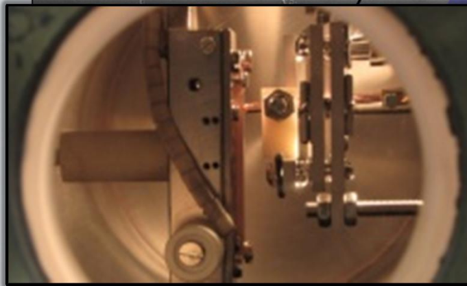
Setup to measure dc sparks on a flat cathode surface (CERN)
