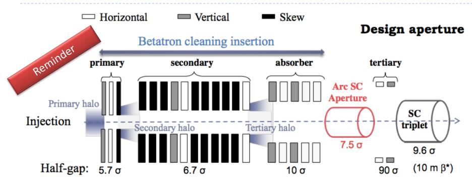
• The protection elements must always be set to an aperture  $\mathbf{a}_{prot} < \mathbf{n}_1$ .
