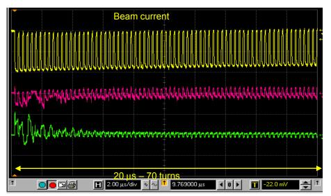
Without the losses from the fast vertical beam instability (plus improved optics control and tuning tools) it is now possible to circulate the 3 A beam with very small losses for hundreds of turns.
