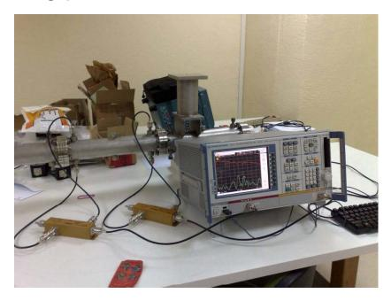
Strip-lines tested up to 3100 V (DC) to ground. Nominal pulse will have about 2800 V. No sparks happened.
