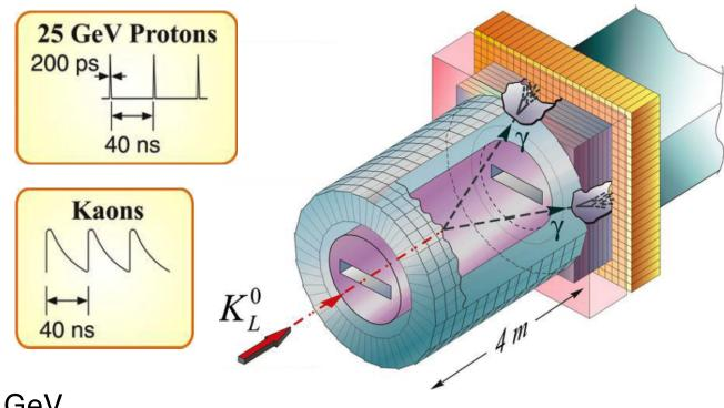
**Microbunched beam from AGS:** Measure  $p(K_L)$  by time of flight 200 ps every 40 ns with  $10^{-3}$  extinction between microbunches
