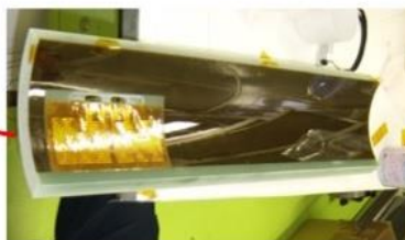
Quench Protection Heaters (LE & RE)
