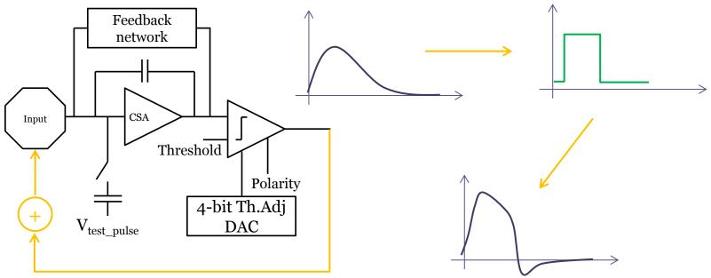
Due to an error in the physical layout of the cell, the output injects charge which feeds back into the input
