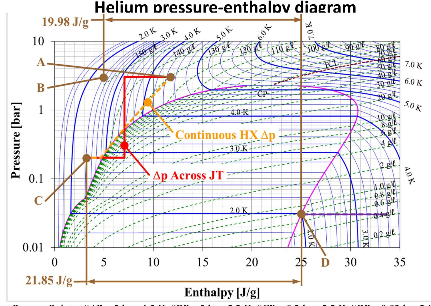
Process Points: "A" = 3 bar, 4.5 K; "B" = 3 bar, 2.2 K; "C" = 0.2 bar, 2.2 K; "D" = 0.03 bar 2.0 K
