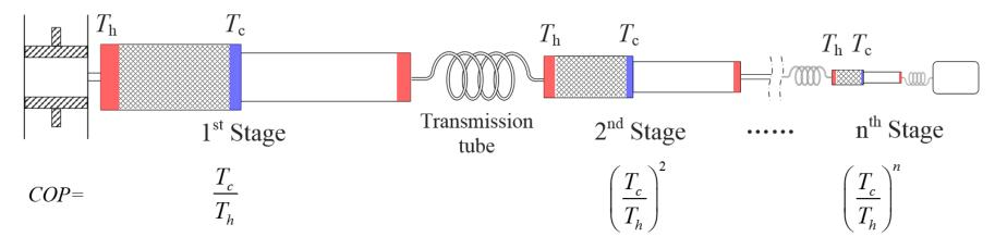
$$Q_{c1} = E_1 \frac{T_c}{T_h} \qquad E_2 = Q_{c1} = E_1 \frac{T_c}{T_h} \qquad Q_{c2} = E_2 \frac{T_c}{T_h} = E_1 \left(\frac{T_c}{T_h}\right)^2 \qquad Q_{cn} = E_{n-1} \frac{T_c}{T_h} = E_1 \left(\frac{T_c}{T_h}\right)^n$$
