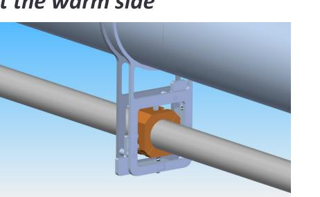
Beam Pipe adjustable support at the cold side
