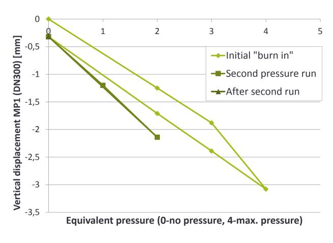
Displacement of the DN300 vertical position (MP1) during the 'burn-in' procedure and the following pressure cycle
