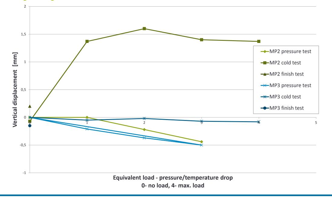
Displacement of the Beam Pipe vertical position at the cold side (MP2) and the warm side (MP3)
