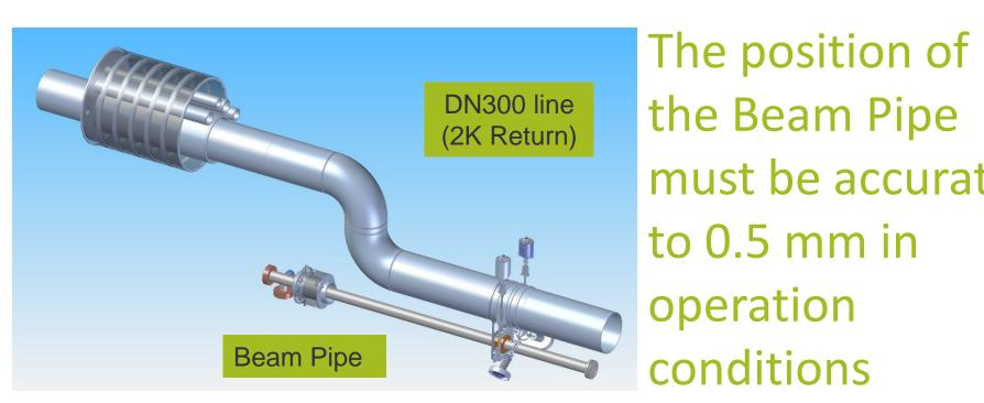
the Beam Pipe must be accurate to 0.5 mm in operation conditions
