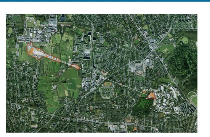
The European XFEL will be located mainly in underground tunnels which can be accessed on three different sites. The 3.4-kilometrelong facility will run from DESY in Hamburg to the town of Schenefeld
