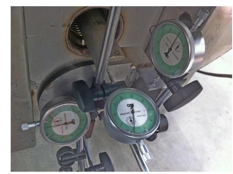
Measuring dial gauge setup Dial gauges for measure the X and Y lisplacements during pressure load and cryogenic thermal cycle test
