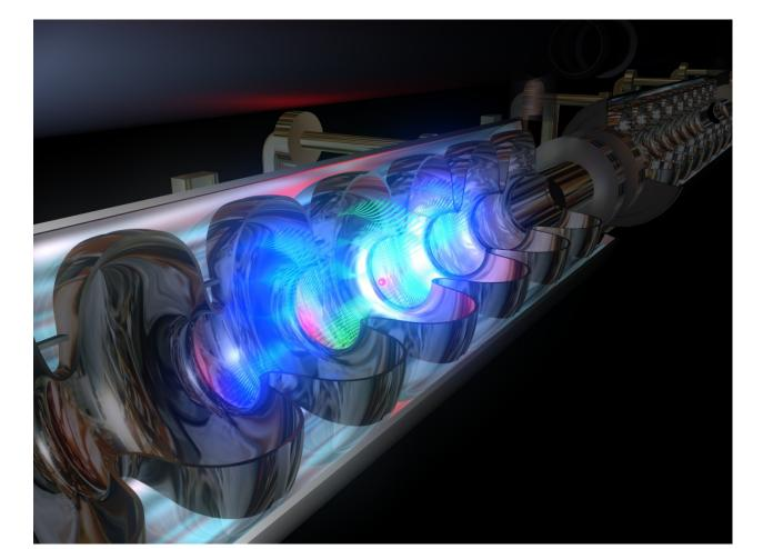
Acceleration in a resonator Electromagnetic fields accelerate the electrons in superconducting resonators
