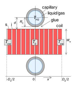
$\Delta T$  between the LH2 and the center of the coil (borrow expression from electrical capacitor)
