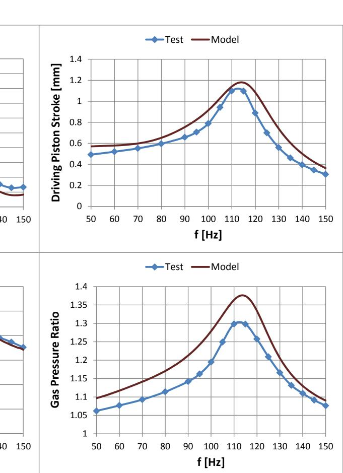
Note: The measurements were taken in the first few seconds from the start of the run; thus, the test system was retained at room temperature, except for the cold heat exchanger of the cryocooler, which was at about 280 K.
