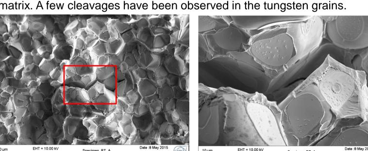
Examination of the fracture surfaces on specimens tested at 77 K revealed a transgranular brittle fracture dominated by cleavage in the tungsten grains. A debounding between them and the matrix is noticed as well.
