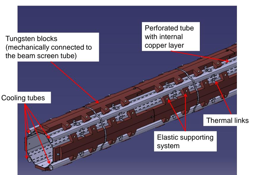
Assembly of the beam screen
