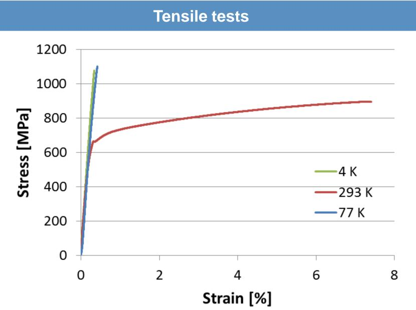
Typical tensile curves of Inermet® 180 at 4.2 K, 77 K and room temperature
