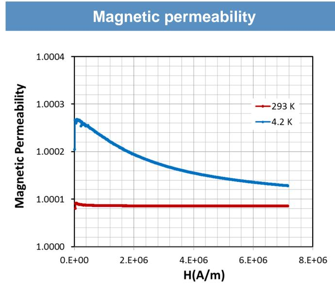
Typical magnetic permeability as a function of magnetic field. Values at room temperature and 4.2K.
