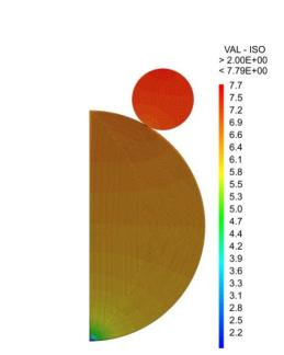
Heat transfer evaluation from the warm beam screen to the cold bore
