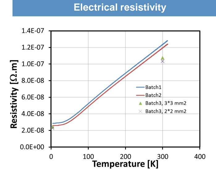
Electrical resistivity as a function of temperature. Batch 1 corresponds to reference number 8017006 and Batch 2 to reference 802482, compare Table 2. The sample dimensions of Batch 1 and 2 have been 2 mm x 2 mm x 73 mm
