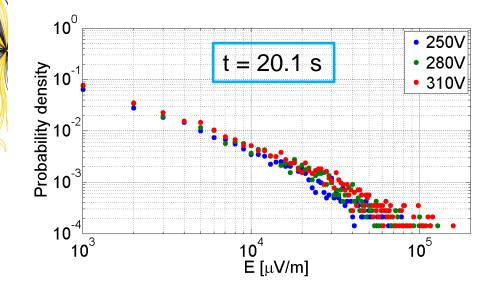
Probability density of  $E_z$  for different pulse amplitudes.
