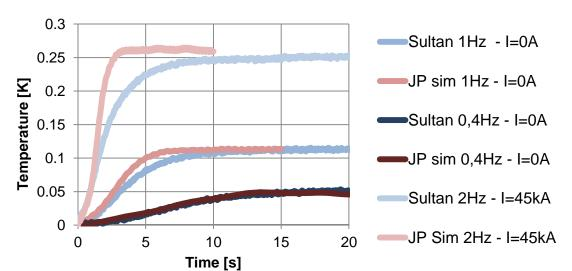
T(t) comparison between JackPot simulations and Sultan measurements for sinusoidal  $B_a$  based on identified  $\rho_{is}$
