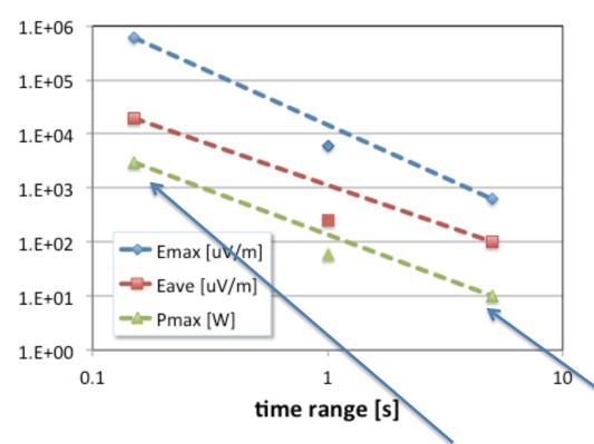
Time scale for pulses are different: for fast sine-wave pulse (0.1 s), 15 MA (1 s),  $T_{cs}$  test (5 s). When simply assuming quasi DC  $T_{cs}$  test as 5 s range and connecting experimental points (power law fit), stable performance is predicted for 15 MA scenario.
