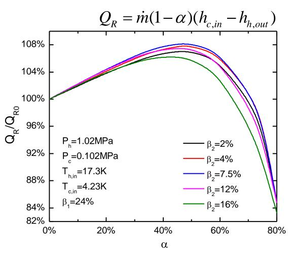
$\beta_2$  indicates the position of bypass and throttling  $\alpha$  indicates the amount of bypass mass
