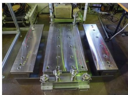
Cryostat stored in an iron core
