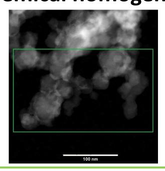
Mass transport diffusion length on 10s of nm scale →ensure homogeneous and synergetic reaction to form Bi2212;
