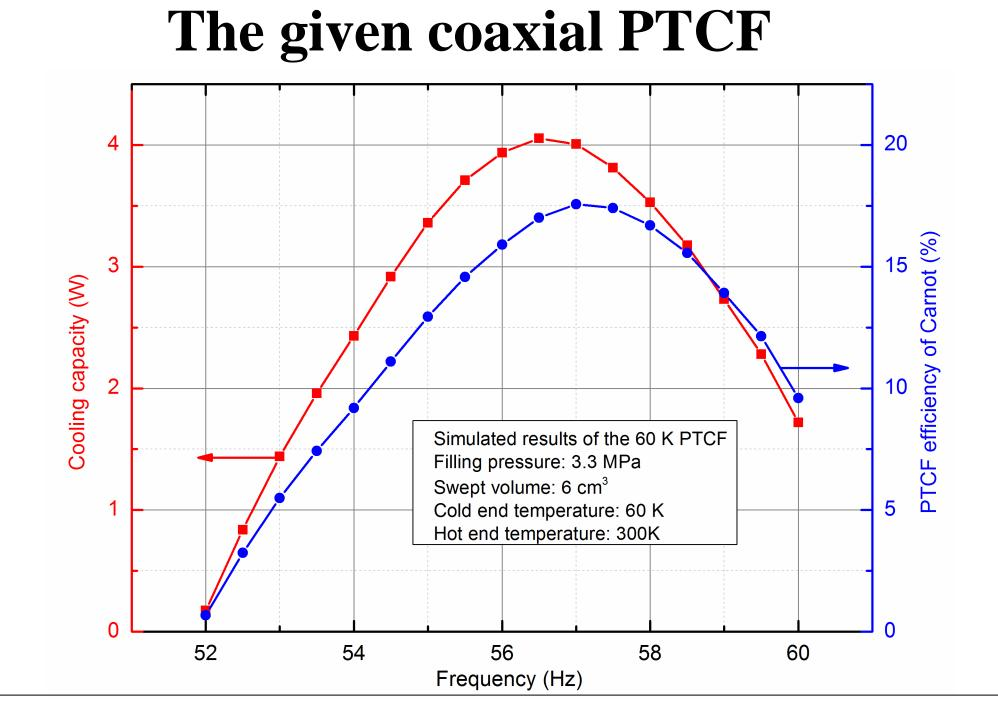
The highest cooling efficiency occurs at the frequency of 57 Hz and the highest cooling capacity occurs at 56.5 Hz.
