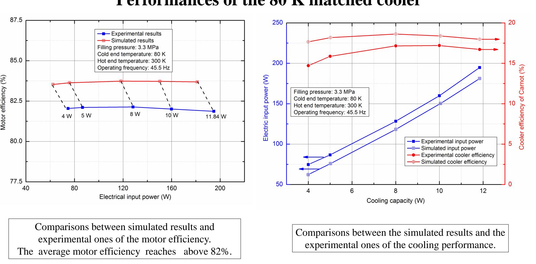
The matched cooler can provide 4 to 11.84 watts at cooling temperature of 80 K with the electrical input power
