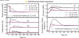
It is found through the simuation results that the feedback heater control approach with  $K_n = 20$  and  $T_i = 10$  could be used without feed-forward control to mitigate the pressure fluctuation for the 600-kW proton beam operation
