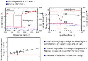
We confirmed that the developed orifice-type heater can apply such a stepwise heat load of kW-order to
