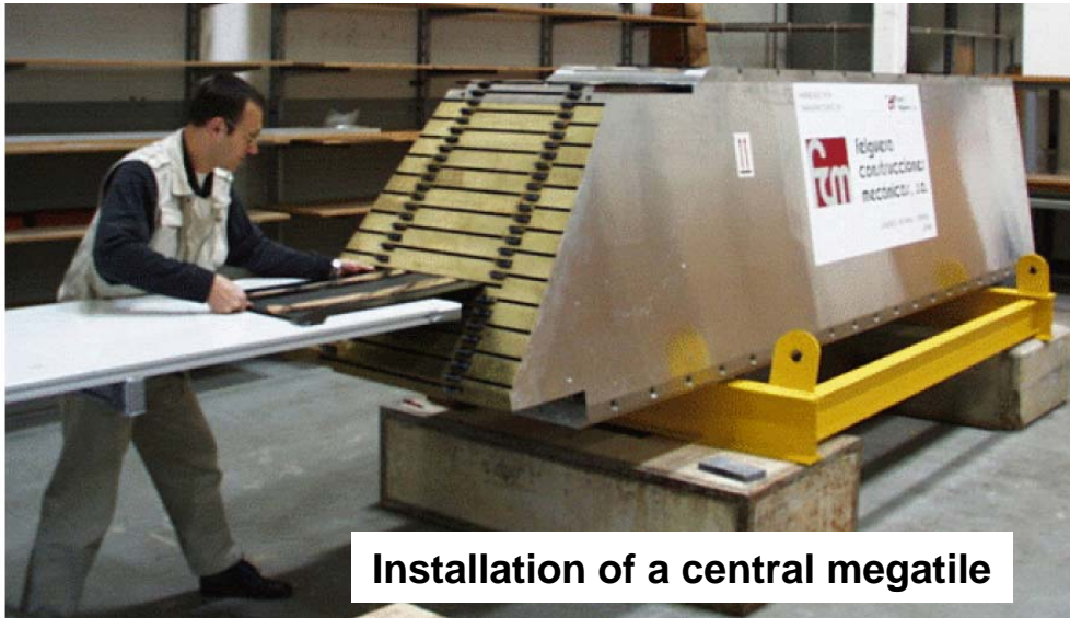
Wave length shift fiber is placed in a groove in each scintillator tile. About 5% of light is captured in the fiber.
