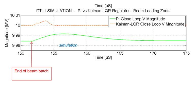
With an improved feedback (Linear Quadratic Regulator, LQG) the transient does not exceed the 1 μs case for any gap length. Feedforward
