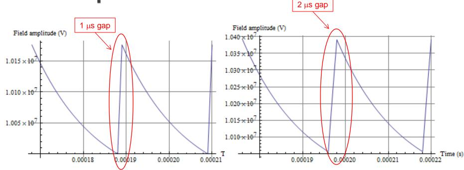
• Effect of a 1 μs and 2 μs gap in the DTL1 voltage (10 MV), without regulation: The voltage increases by ~ 2% and 4% respectively. 40 mA DC beam current.
