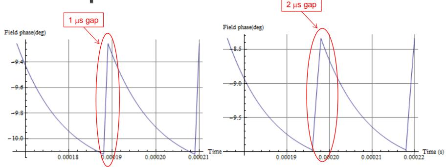
• Effect of a 1 μs and 2 μs gap in the Buncher, without regulation (150 kV): The phase drifts by  $\sim$  0.8 deg. and 1.6 deg. respectively. 40 mA DC beam current.
