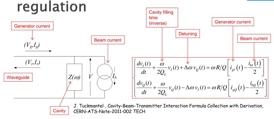
Transients in the beam current result in transients in the cavity field (amplitude and phase).
