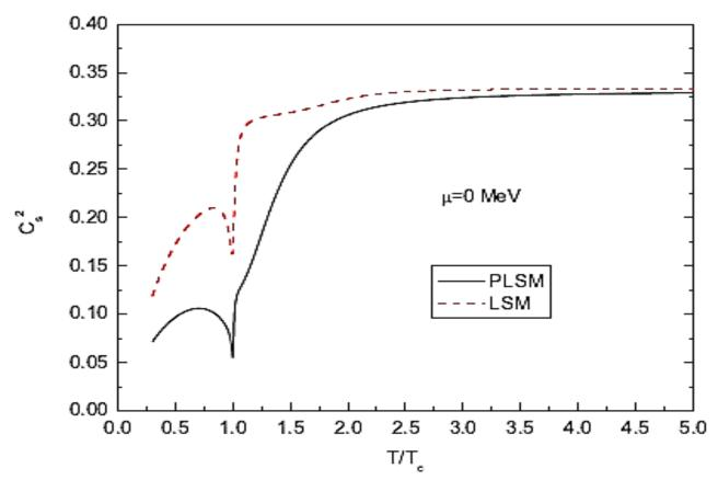
In conformal field theories including free field theory, the squared speed of sound is 1/3. Near  $T_c \rightarrow$  downward cusp. At zero density,  $\rightarrow$  minimum
