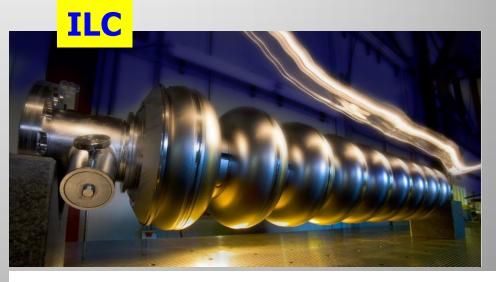
Superconducting RF cavities (like XFEL)
