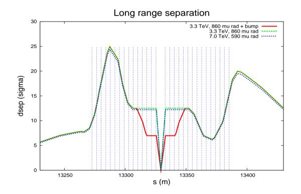
→ decreased separation near IP, smaller "effective" angle ⇒ geometric loss much reduced (± 240  $\mu$ rad, ≈ 40% more)
