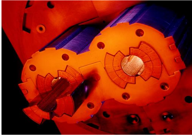
NbTi LHC standard dipoles, 8.3 T
