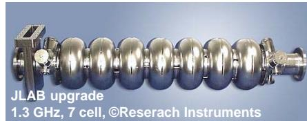
SC RF allows to built an ERL “compact” (high gradient) for high current cw operation (large apertures, strong HOM damping)
