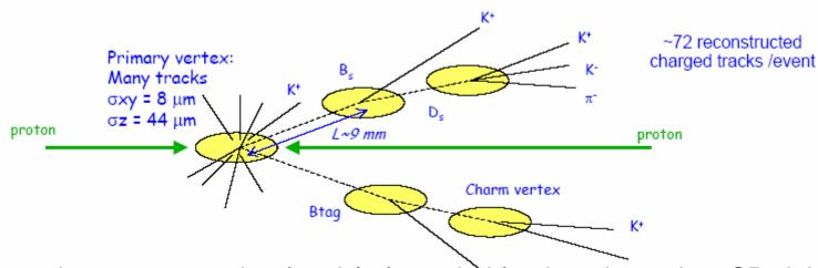
Proper time reconstruction (t=mL/pc) needed for time dependant CP violation measurements: need to measure L(~9mm) and p (~1-100 GeV/c) , resolution ~ 40 fs (B<sub>s</sub>  $\rightarrow$  D<sub>s</sub>- $\pi$ +)
