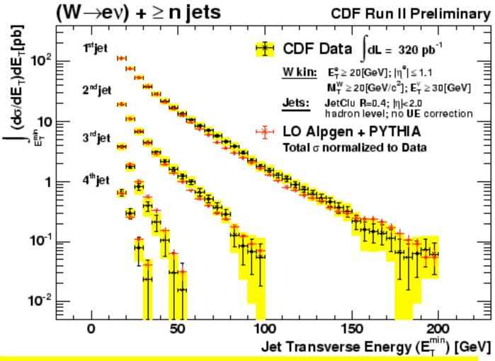
MC has been normalized to inclusive data cross section in each jet sample!
