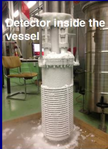
10x10x20 cm LEM-anode fast test setup
