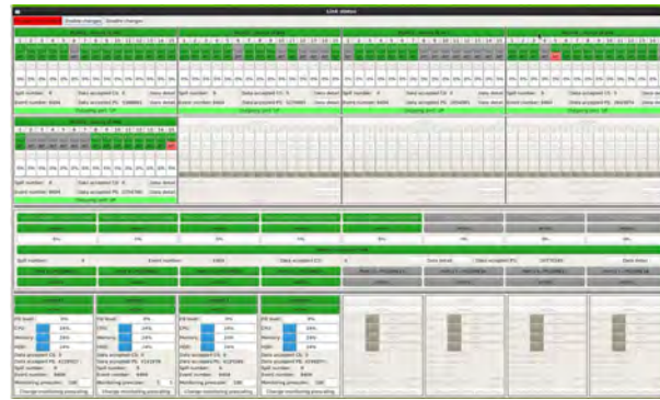
Fig. 56: The Interactive status and configuration GUI shows status of all attached front-end modules, DAQ modules and Readout Engine computers.
