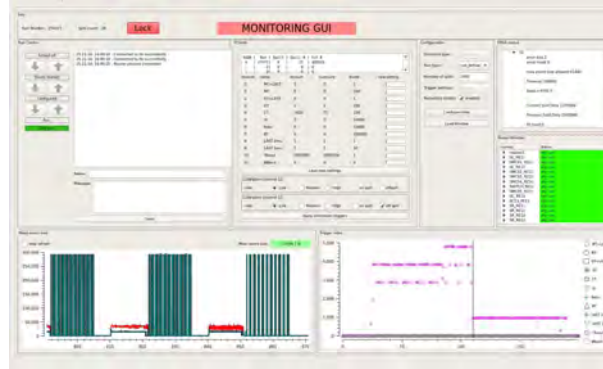
Fig. 55: The Run Control GUI displays status of the DAQ, trigger rates, prescaling values and event sizes ver
