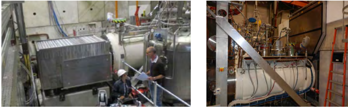
Fig. 44: The fully assembled hadron absorber in the COMPASS hall: (left) before and (right) after the installation of the concrete shielding and Vertex Detector.
