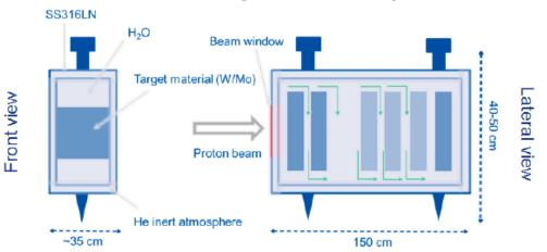
Pressurized water cooling of 15-20 bar
