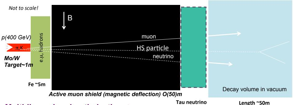
Multidimensional optimization: beam energy, Detector ~10m beam intensity, background conditions and detector acceptance
