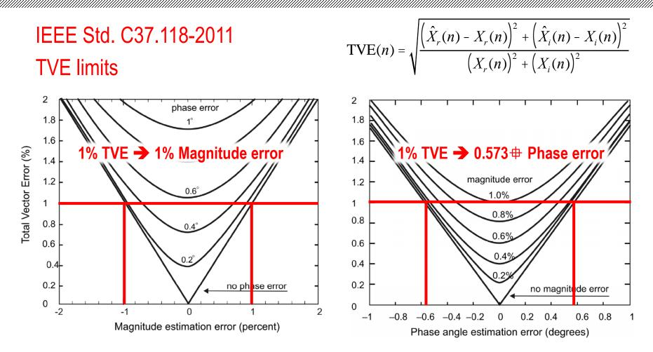
Is a 1% TVE-compliant PMU sufficiently accurate to allow its use in Active Distribution Networks (ADNs)?
