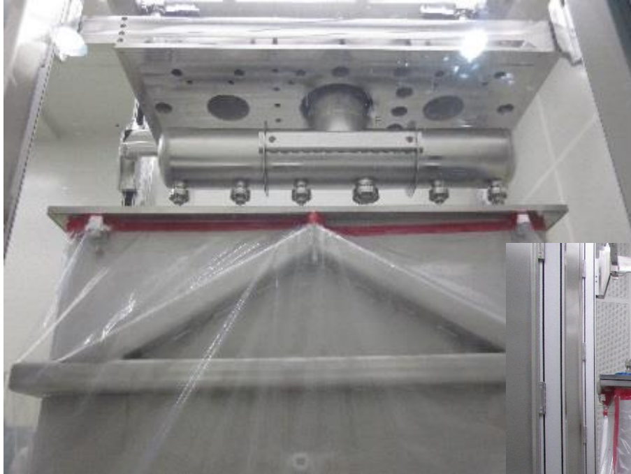
Insertion test and vacuum leak test
