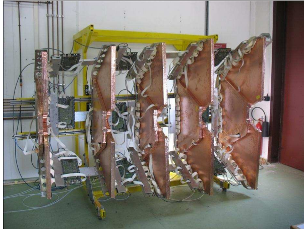
Figure 2: One quarter of the T1 telescope mounted on its support structure.
