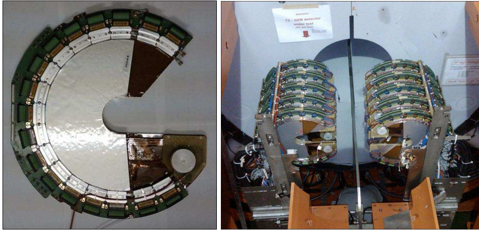
Figure 3: Left: GEM chamber assembled with its horseshoe-shaped readout card. Right: One arm of the T2 telescope just before the insertion in the CMS HF calorimeter.
