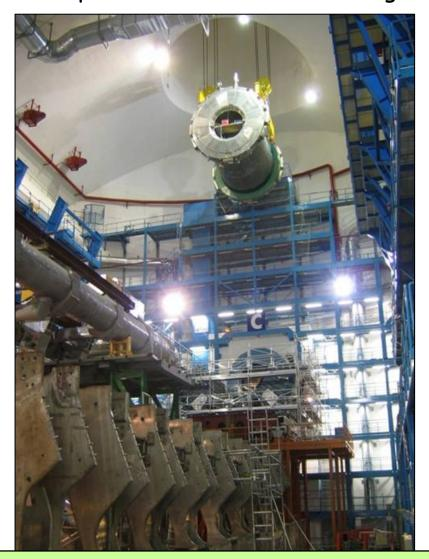
Pb-liquid argon sampling calorimeter with Accordion shape, covering  $|\eta|$  < 2.5
