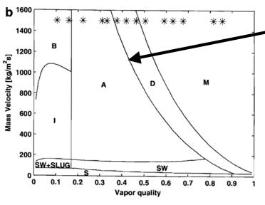
As the mass flux increases, dryout occurs at lower and lower vapor fractions
