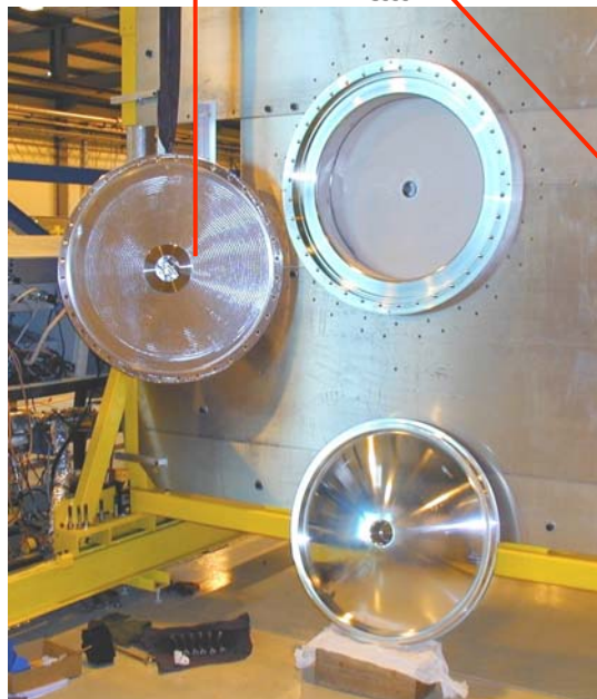
Al exit window of VELO tank
