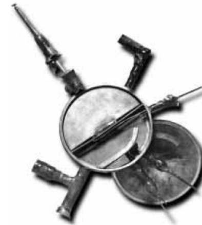
Ernest Lawrence's first successful cyclotron, built in 1930. It was 13 cm in diameter and accelerated protons to 80 keV
