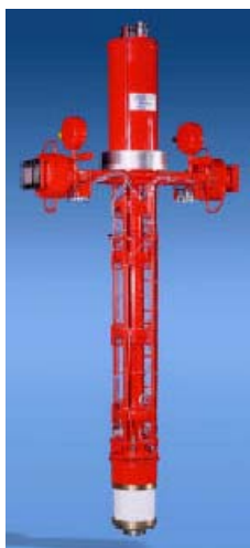
Thales MBK TH1801 10 MW, 1.3 GHz (measured)
